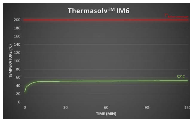
Figure 7. IM6 cooling performances with a heat source
